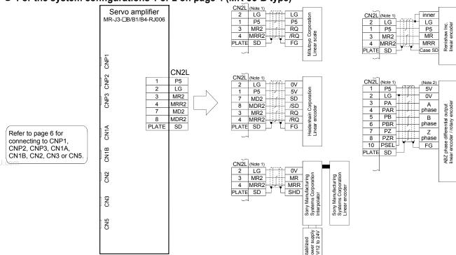
Notes: 1. When manufacturing the linear encoder connection cable, use the optional CN2L connector (MR-J3CN2). Refer to "MR-J3-□B-RJ006 SERVO AMPLIFIER INSTRUCTION MANUAL" for details on the wiring.
