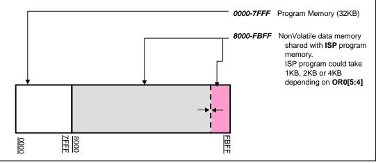
Address Space for MPC89E58A embedded Flash memory
