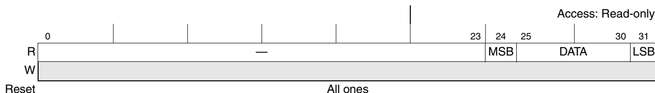
Figure 19-13. Example SPMODE[REV] = 1 SPMODE[LEN] = 7 MSB Sent First
