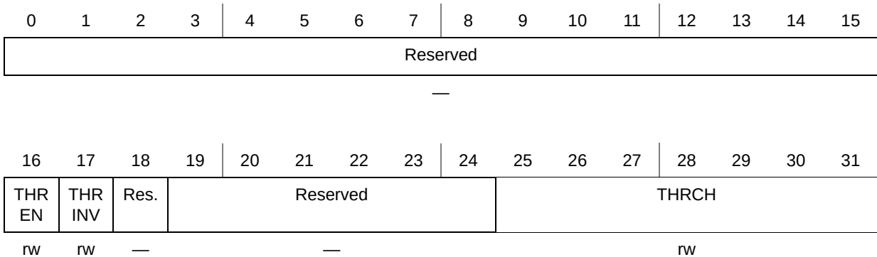
Figure 5-15. Threshold Control Register (TRCx, x = [0..3])
