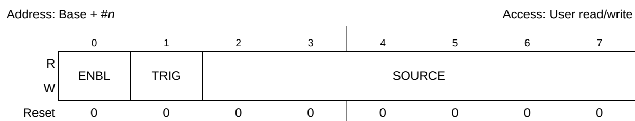
Figure 16-2. Channel Configuration Registers (CHCONFIG#n)
