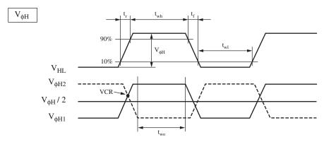
The overlap period of  $t_{wh}$  of horizontal transfer pulse  $V_{\phi H1}$  and  $t_{wl}$  of  $V_{\phi H2}$  and the overlap period of  $t_{wl}$ of horizontal transfer pulse  $V_{\varphi H1}$  and  $t_{wh}$  of  $V_{\varphi H2}$  are defined as  $t_{wo}$ . And VCR is the cross point voltage of the rising  $V_{\varphi H1}$  and the falling  $V_{\varphi H2}$ .
