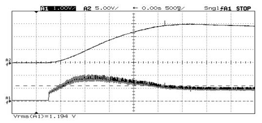
In the second plot we directly connect the same motor to the line voltage:
