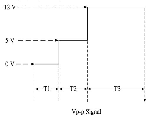
The voltage, waveform and timing requirments for VPP to program IC are as followed:
