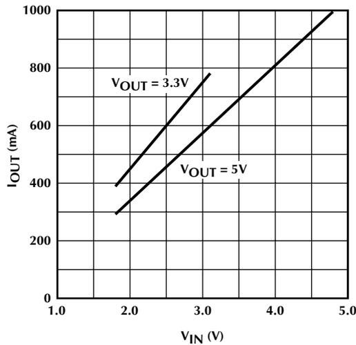
Figure 4. I<sub>OUT</sub> vs. V<sub>IN</sub> Using the Circuit of Figure 8
