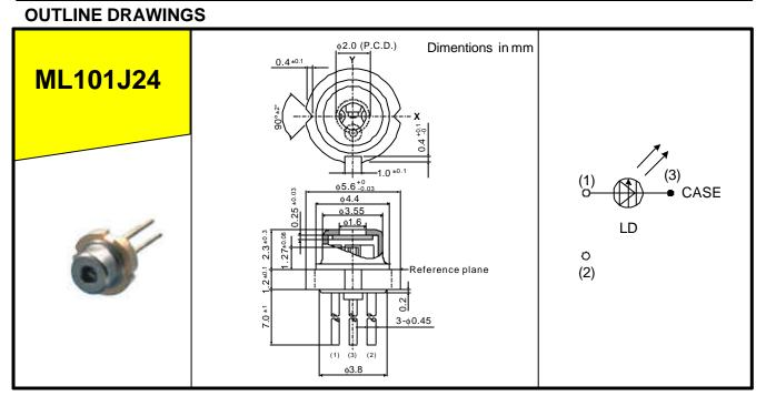
There is no model with a monitor photo diode in ML1XX24 series.
