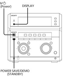
→ Press POWER SAVE/DEMO (STANDBY) when the power is off. The system switches to the Power Saving Mode and the clock display disappears. The system is powering on/off by pressing I/<sup>(1)</sup>.
