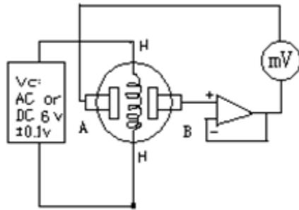
Sensor testing circuit pic. The resistance in this testing circuit should be greater than 100 GΩ, otherwise it would affect the sensor performance.
