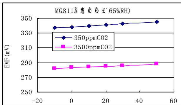
**Fig5. Typical temperature characteristics**
