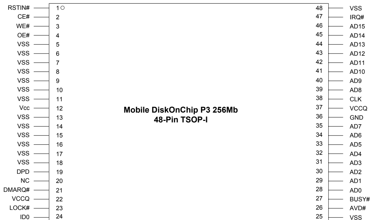
Figure 4: Pinout for Multiplexed Interface (Mobile DiskOnChip P3 256Mb TSOP-I Package)
