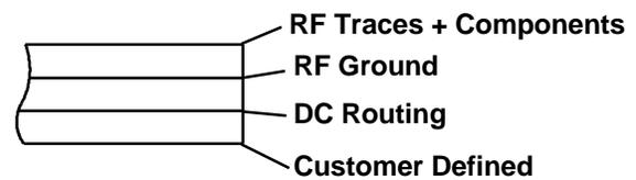
The PCB dielectric between RF traces and RF ground layers should be chosen to reduce RF discontinuities between 50Ω lines and package pins. M/A-COM recommends an FR-4 dielectric thickness of 0.008" (0.2 mm) yielding a 50Ω line width of 0.015" (0.38 mm). The recommended metalization thickness is 1 ounce copper.
