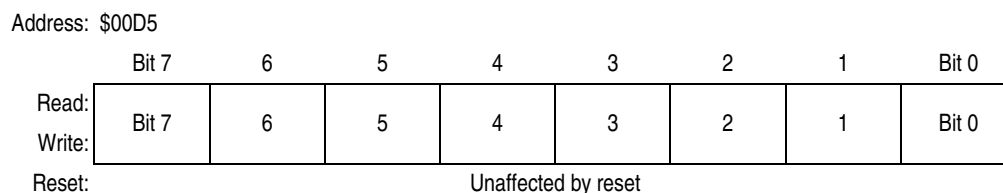
Figure 15-13. SPI Data Register (SP0DR)
