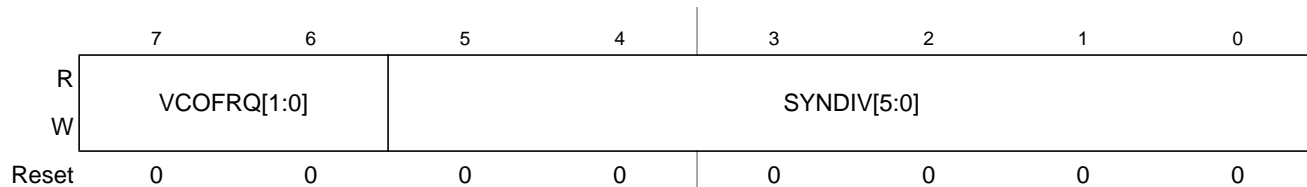
Figure 7-3. S12XECRG Synthesizer Register (SYNR)
