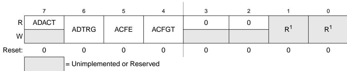
Figure 9-5. Status and Control Register 2 (ADCSC2)
