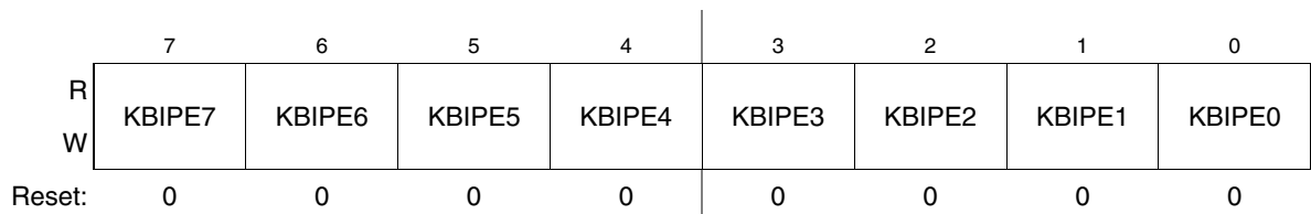
Figure 7-3. KBI Pin Enable Register (KBIPE)
