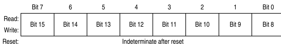
Figure 14-12. TIM Channel x Register High (TCHxH)
