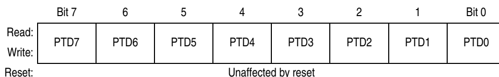
Figure 11-13. Port D Data Register (PTD)
