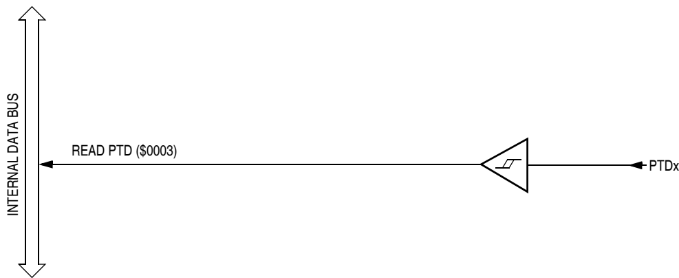
Figure 15-12. Port D Input Circuit
