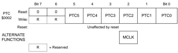
Figure 19-7. Port C Data Register (PTC)
