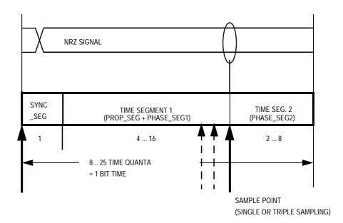
Figure 20-8. Segments Within the Bit Time
