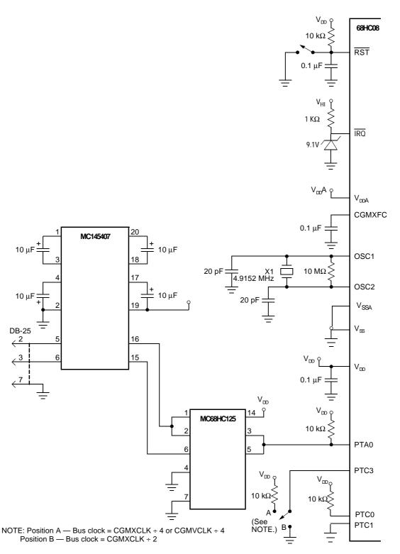
Figure 11-1. Monitor Mode Circuit
