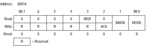
Figure 14-3. IRQ Status and Control Register (ISCR)
