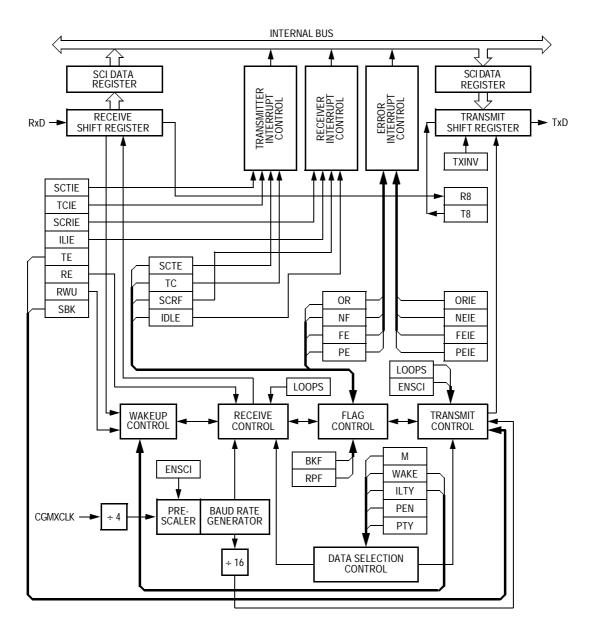
Figure 15-1. SCI Module Block Diagram
