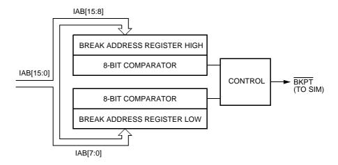
Figure 10-1. Break Module Block Diagram
