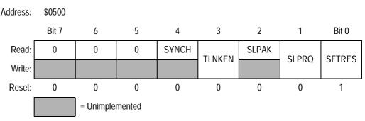
Figure 20-15. Module Control Register 0 (CMCR0)
