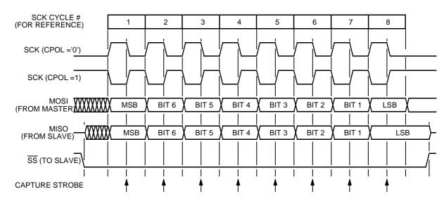
Figure 16-5. Transmission Format (CPHA = '1')
