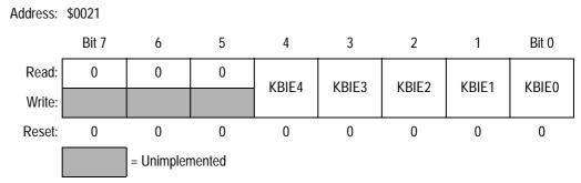
Figure 21-4. Keyboard Interrupt Enable Register (KBIER)
