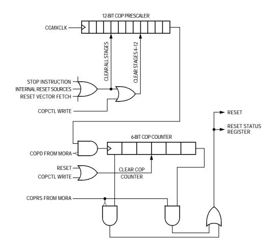
Figure 12-1. COP Block Diagram
