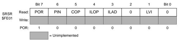
Figure 7-16. SIM Reset Status Register (SRSR)
