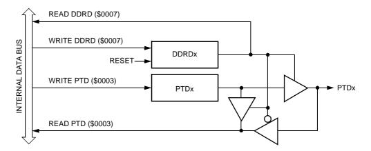
Figure 19-12. Port D I/O Circuit
