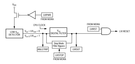
Figure 13-1. LVI Module Block Diagram
