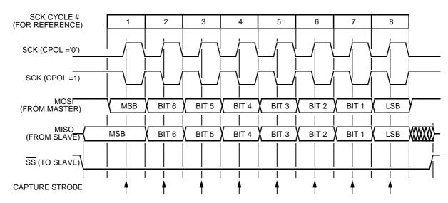
Figure 16-4. Transmission Format (CPHA = '0')
