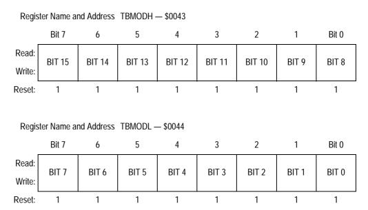
Figure 17-6. TIMB Counter Modulo Registers (TBMODH and TBMODL)
