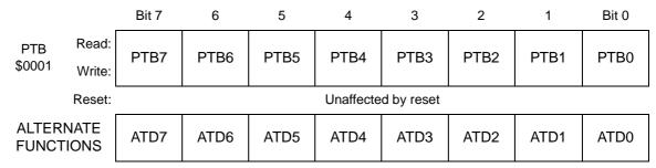
Figure 19-4. Port B Data Register (PTB)
