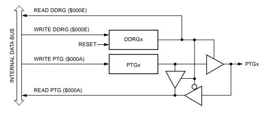
Figure 19-21. Port G I/O Circuit
