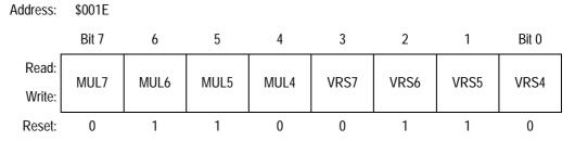
Figure 8-6. PLL Programming Register (PPG)
