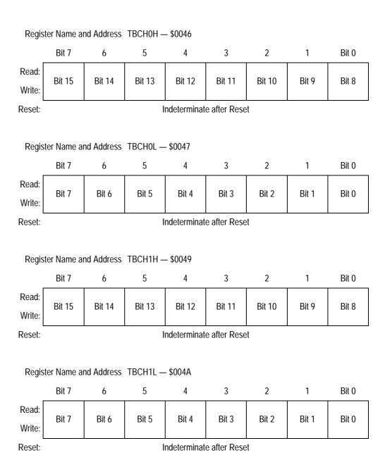
Figure 17-9. TIMB Channel Registers (TBCH0H/L-TBCH1H/L)
