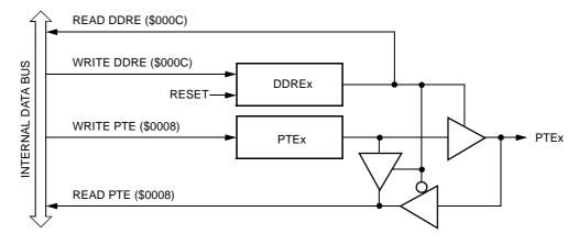
Figure 19-15. Port E I/O Circuit
