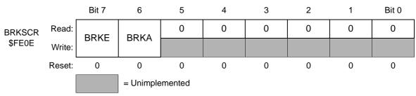
Figure 10-2. Break Status and Control Register (BRKSCR)
