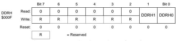
Figure 19-23. Data Direction Register H (DDRH)
