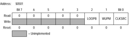
Figure 20-16. Module Control Register (CMCR1)
