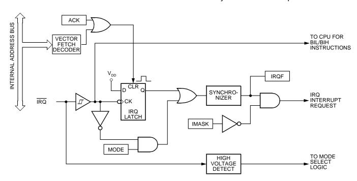
Figure 14-1. IRQ Module Block Diagram
