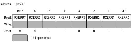
Figure 20-24. Receiver Error Counter (CRXERR)
