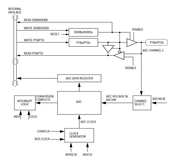
Figure 23-1. ADC Block Diagram
