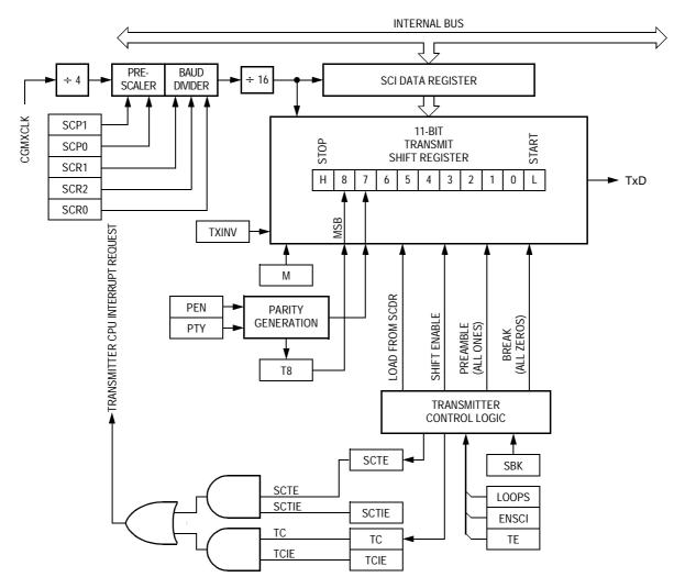
Figure 15-4. SCI Transmitter
