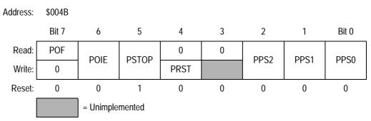
Figure 18-3. PIT Status and Control Register (PSC)
