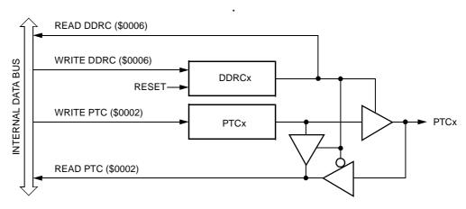
Figure 19-9. Port C I/O Circuit
