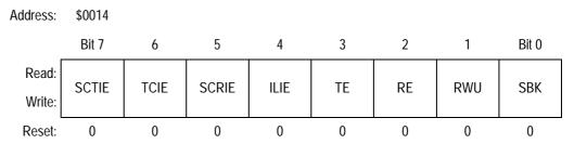
Figure 15-12. SCI Control Register 2 (SCC2)
