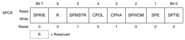
Figure 16-12. SPI Control Register (SPCR)
