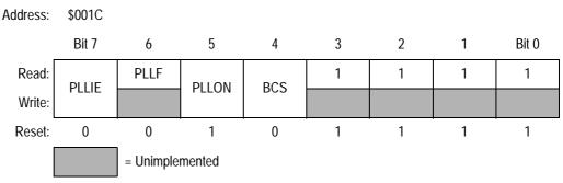
Figure 8-4. PLL Control Register (PCTL)
