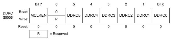
Figure 19-8. Data Direction Register C (DDRC)
