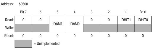
Figure 20-23. Identifier Acceptance Control Register (CIDAC)
