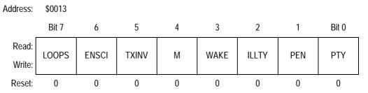
Figure 15-11. SCI Control Register 1 (SCC1)
