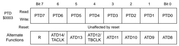
Figure 19-10. Port D Data Register (PTD)
