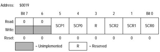
Figure 15-18. SCI Baud Rate Register (SCBR)
