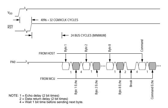
Figure 11-6. Monitor Mode Entry Timing
