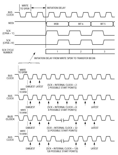
Figure 16-6. Transmission Start Delay (Master)
