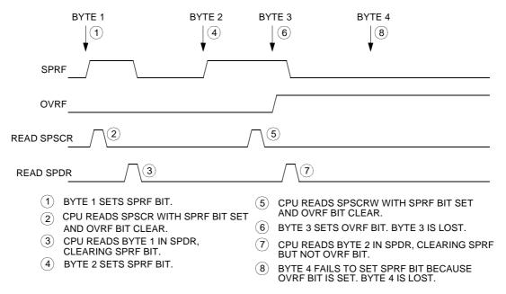
Figure 16-7. Missed Read of Overflow Condition
