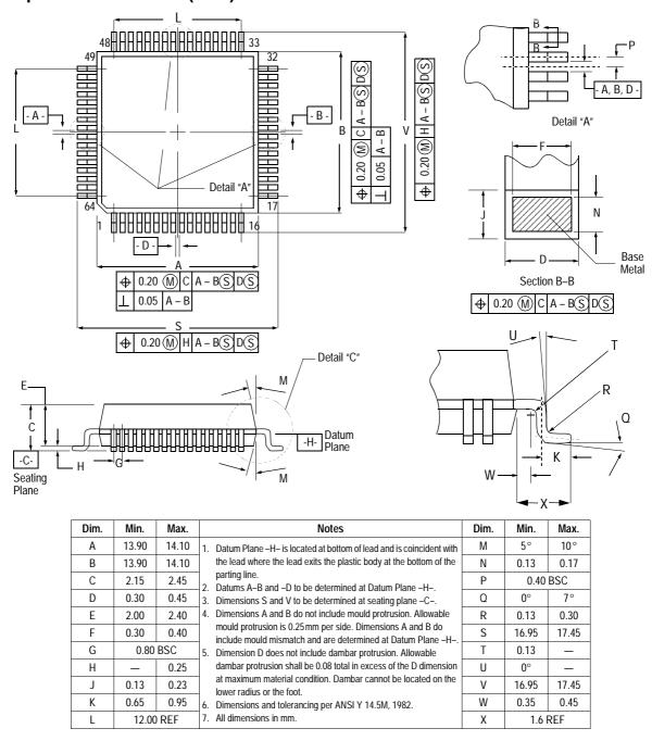
Figure 24-3. 64-pin QFP (Case #840B)
