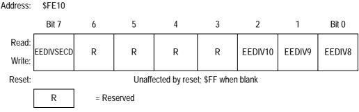
Figure 5-7. EEPROM Divider Non-Volatile Register High (EEDIVHNVR))
