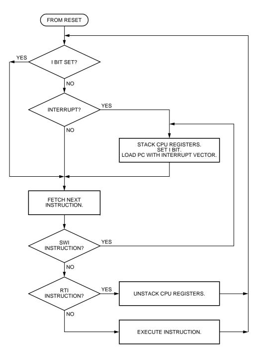
Figure 14-2. IRQ Interrupt Flowchart
