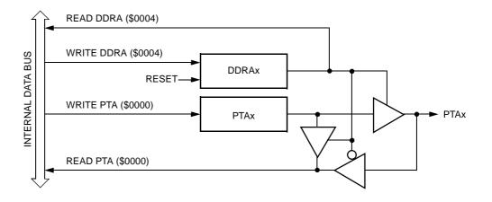
Figure 19-3. Port A I/O Circuit
