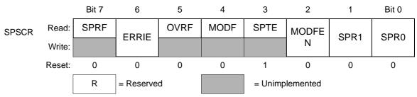
Figure 16-13. SPI Status and Control Register (SPSCR)
