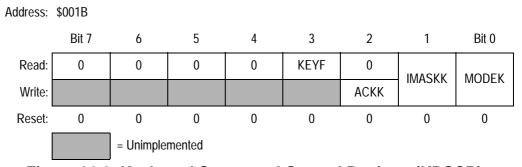
Figure 21-3. Keyboard Status and Control Register (KBSCR)
