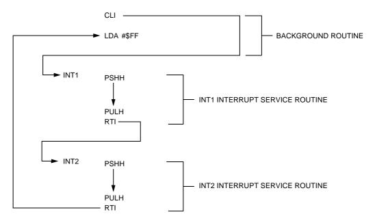
Figure 7-9. Interrupt Recognition Example
