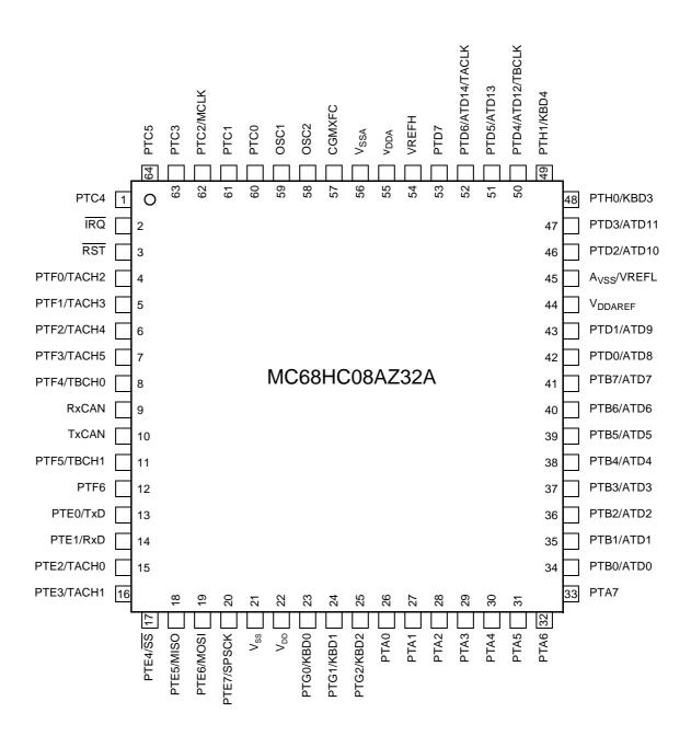
Figure 1-2. 64 QFP Pin Assignments
