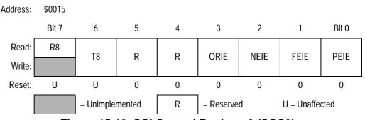
Figure 15-13. SCI Control Register 3 (SCC3)
