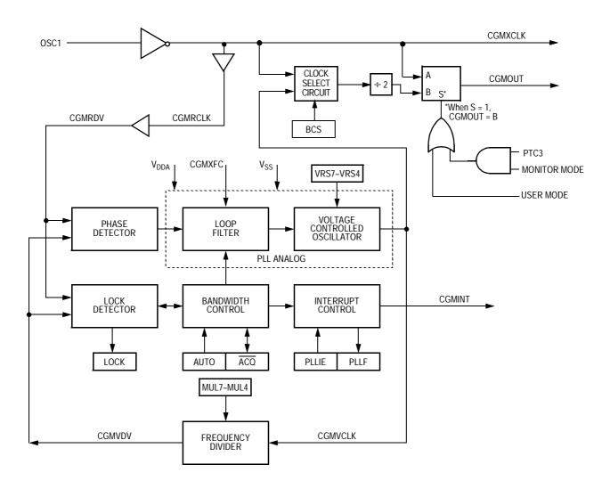
Figure 8-1. CGM Block Diagram
