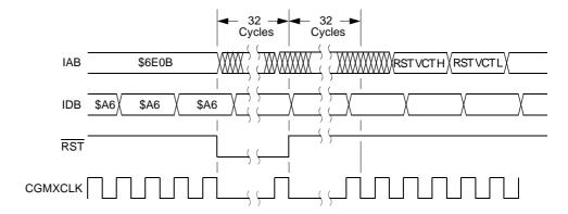
Figure 7-12. WAIT Recovery From Internal Reset
