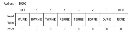
Figure 20-20. Receiver Interrupt Enable Register (CRIER)
