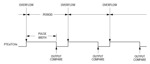
Figure 22-3. PWM Period and Pulse Width
