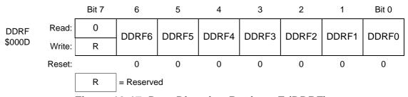
Figure 19-17. Data Direction Register F (DDRF)
