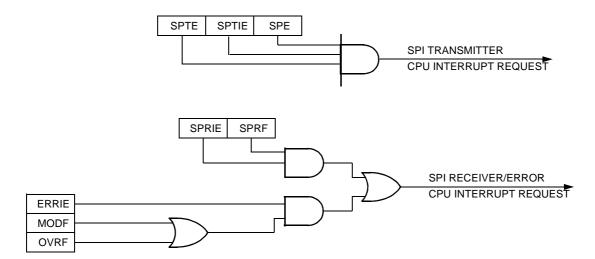
Figure 16-9. SPI Interrupt Request Generation
