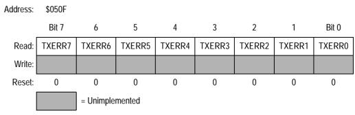
Figure 20-25. Transmit Error Counter (CTXERR)
