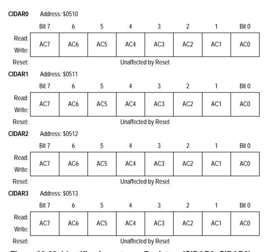
Figure 20-26. Identifier Acceptance Registers (CIDAR0-CIDAR3)
