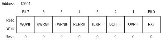
Figure 20-19. Receiver Flag Register (CRFLG)
