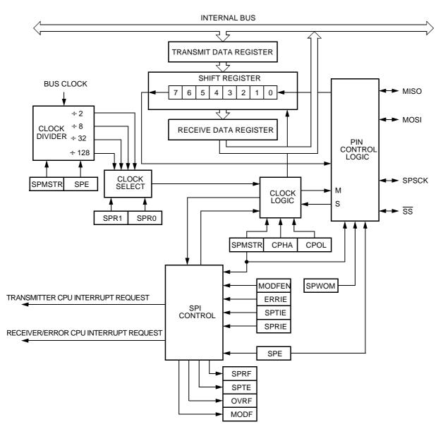
Figure 16-2. SPI Module Block Diagram
