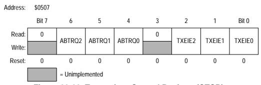
Figure 20-22. Transmitter Control Register (CTCR)
