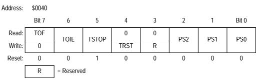
Figure 17-4. TIMB Status and Control Register (TBSC)
