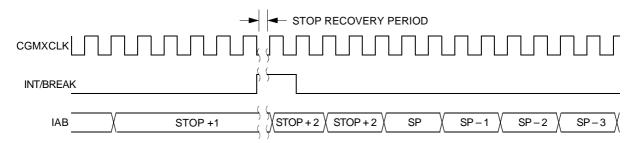
Figure 7-14. STOP Mode Recovery From Interrupt
