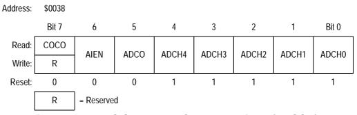
Figure 23-2. ADC Status and Control Register (ADSCR)
