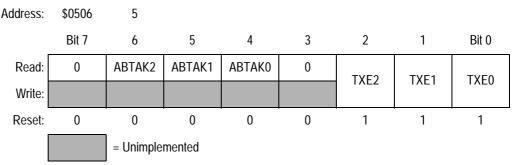
Figure 20-21. Transmitter Flag Register (CTFLG)
