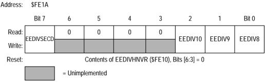
Figure 5-5. EEDIV Divider High Register (EEDIVH)
