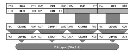
Figure 20-3. Single 32-Bit Maskable Identifier Acceptance Filter
