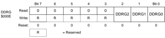
Figure 19-20. Data Direction Register G (DDRG)
