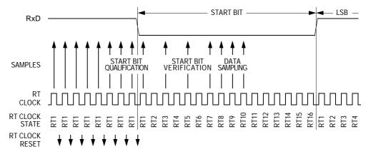
Figure 15-8. Receiver Data Sampling
