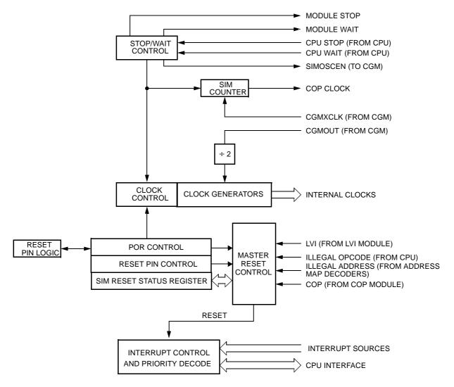
Figure 7-1. SIM Block Diagram
