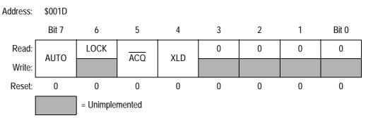
Figure 8-5. PLL Bandwidth Control Register (PBWC)
