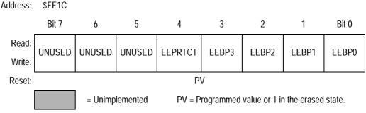
Figure 5-4. EEPROM Nonvolatile Register (EENVR)
