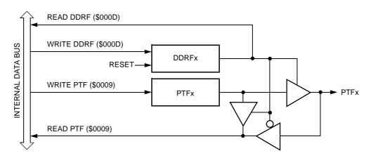
Figure 19-18. Port F I/O Circuit
