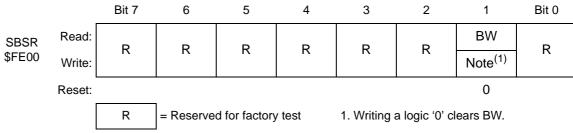
Figure 7-15. SIM Break Status Register (SBSR)
