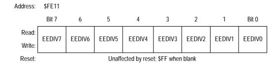
Figure 5-8. EEPROM Divider Non-Volatile Register Low (EEDIVLNVR)
