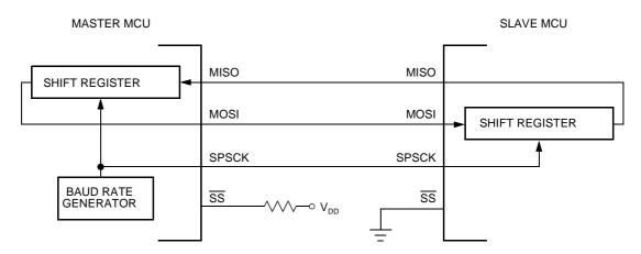
Figure 16-3. Full-duplex Master-Slave Connections
