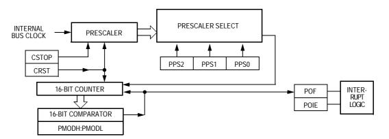
Figure 18-1. PIT Block Diagram
