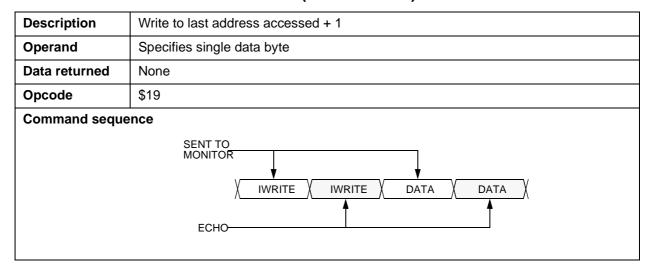
A sequence of IREAD or IWRITE commands can sequentially access a block of memory over the full 64K byte memory map.
