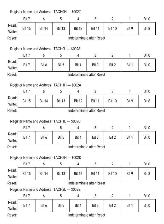
Figure 22-9. TIMA Channel Registers (TACH0H/L-TACH5H/L) (Sheet 1 of 2)
