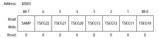
Figure 20-18. Bus Timing Register 1 (CBTR1)
