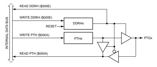
Figure 19-24. Port H I/O Circuit
