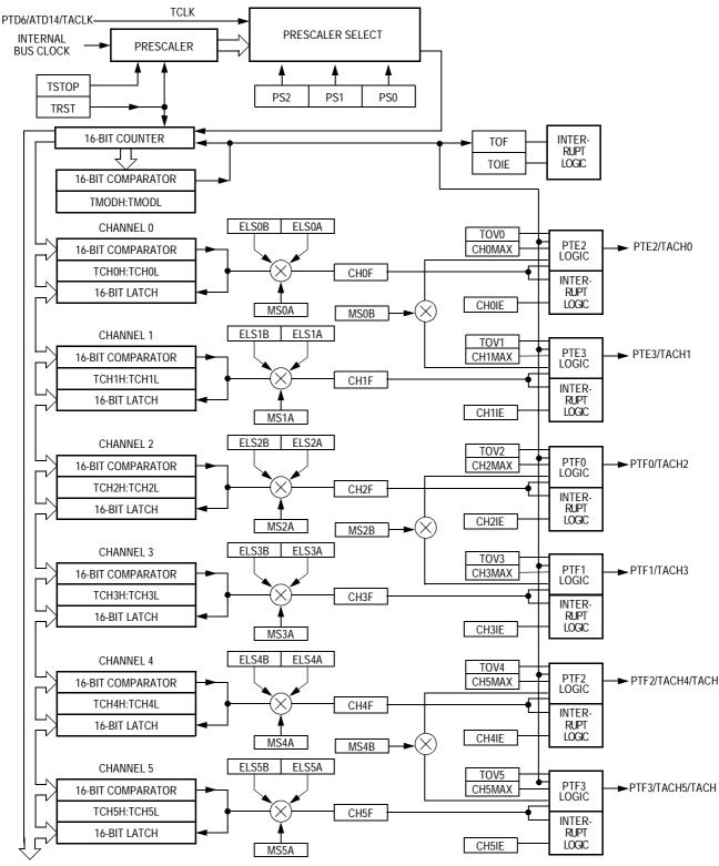
Figure 22-1. TIMA Block Diagram
