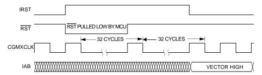
Figure 7-4. Internal Reset Timing
