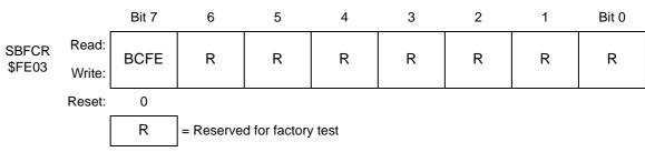
Figure 7-17. SIM Break Flag Control Register (SBFCR)
