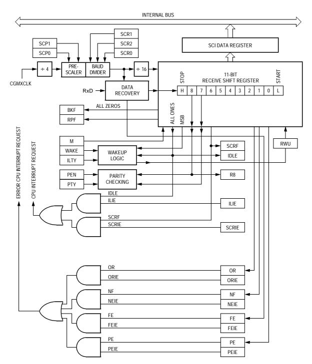
Figure 15-6. SCI Receiver Block Diagram
