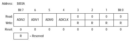
Figure 23-4. ADC Input Clock Register (ADICLK)
