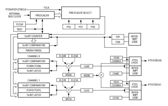
Figure 17-1. TIMB Block Diagram
