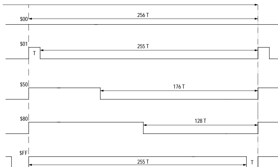
Figure 12-2 PWM output waveforms (POL = 1, active high)
