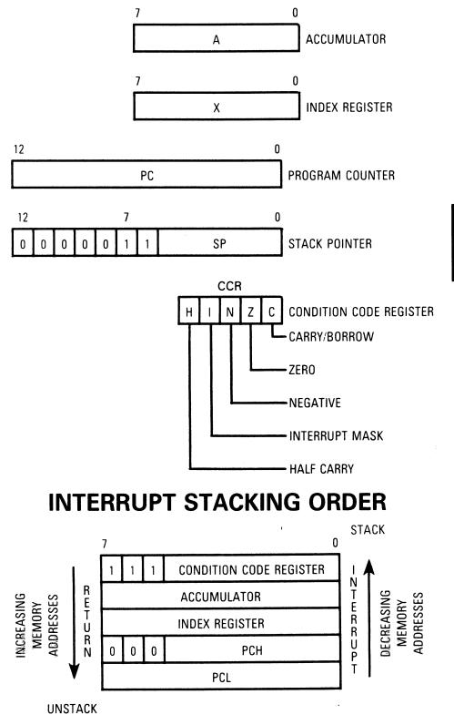
NOTE: Since the Stack Pointer decrements during pushes, the PCL is stacked firstof and the first of the stack is in the reverse order. Go to: www.freescale.com
