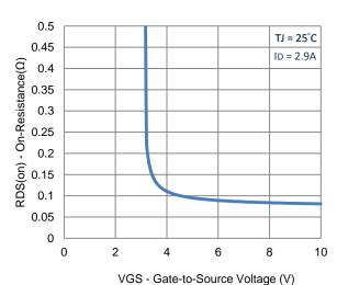
3. On-Resistance vs. Gate-to-Source Voltage
