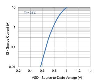
4. Drain-to-Source Forward Voltage
