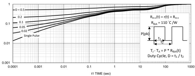
11. Normalized Thermal Transient Junction to Ambient
