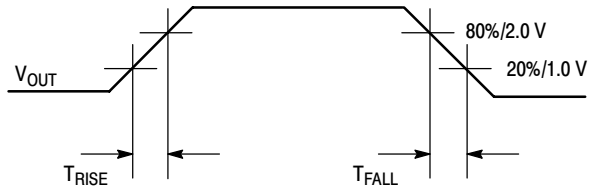
Figure 5. WAVEFORMS: Rise and Fall Times
