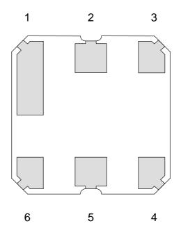
TERMINAL 2: INPUT 5: OUTPUT 1,3,4,6: GROUND **OKI** Semiconductor **MBF9402B**
