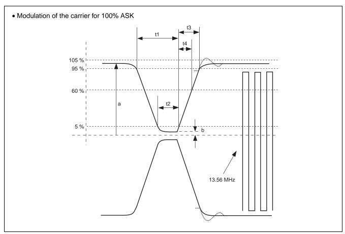
Maximum and minimum values of t1, t2 and t3 are specified in "■ RECOMMENDED OPERATION CONDITIONS". y is 0.05 (a-b) and the maximum value of hf and hr is 0.1(a-b).
