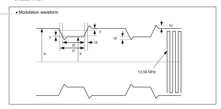
Maximum and minimum values of t1, t2 and t3 are shown in the following table. In this table, y is 0.05 (a-b) and the maximum value of hf and hr is 0.1(a-b).
