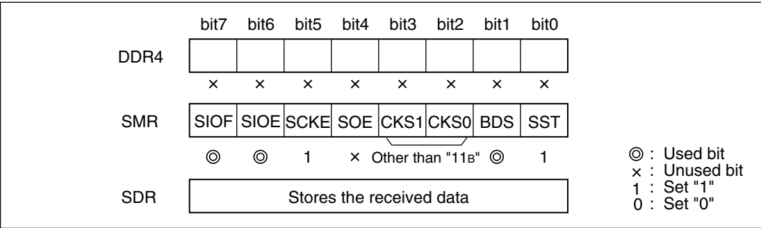
Figure 18.7-1 Serial Input Settings (for an Internal Shift Clock)
