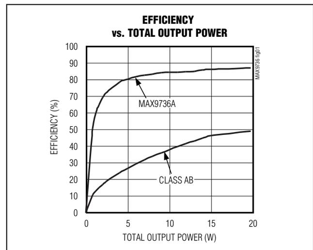
Figure 1. MAX9736A Efficiency vs. Class AB Efficiency
