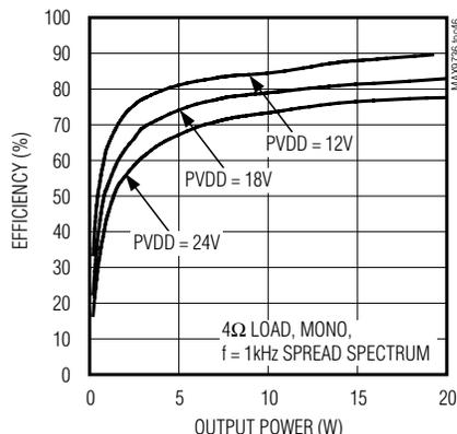
**OUTPUT POWER vs. V<sub>DD</sub> (LOAD = 4Ω, f = 1kHz, SPREAD SPECTRUM, MONO)**
