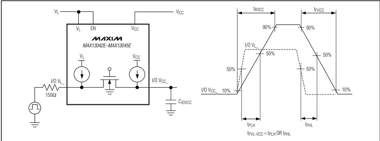
Figure 1. Push-Pull Driving I/O V<sub>L</sub>- Test Circuit and Timing
