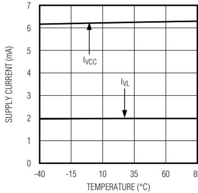
**SUPPLY CURRENT vs. TEMPERATURE (DRIVING ONE I/O  $V_L$ )**
