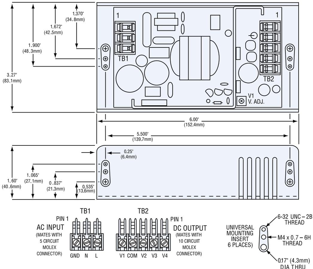
**INPUT & OUTPUT CONNECTIONS:** 6-32 SCREW WIRE CLAMPS ON 0.312" (7.9mm) CENTERS, 0.045" (1.1mm) SQUARE PINS ON 0.156" (3.4mm) CENTERS, MATES WITH MOLEX SERIES 2139, 6442, OR 41695
