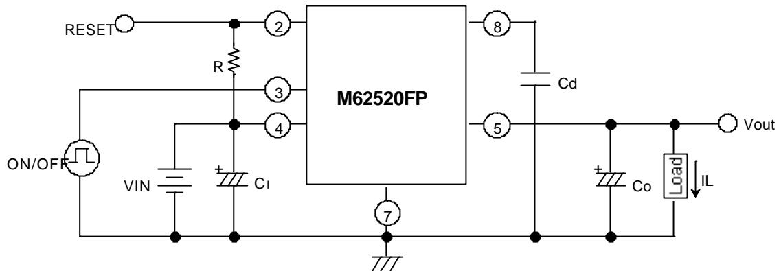
Note1. R is a pull-up resistance for reset terminal. 2.2kohm is recommended for the value.
