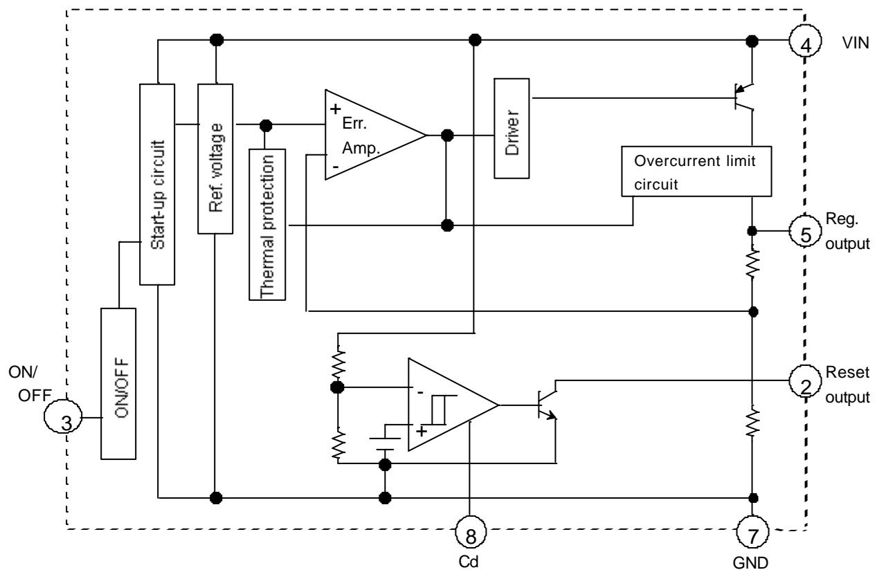
**PRELIMINARY****M62520FP**HIGH PRECISION LOW INPUT/OUTPUT DIFFERENTIAL 3.3V FIXED
