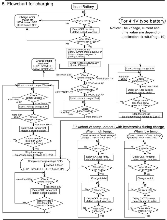
Charge Control IC for Li-Ion Batteries
