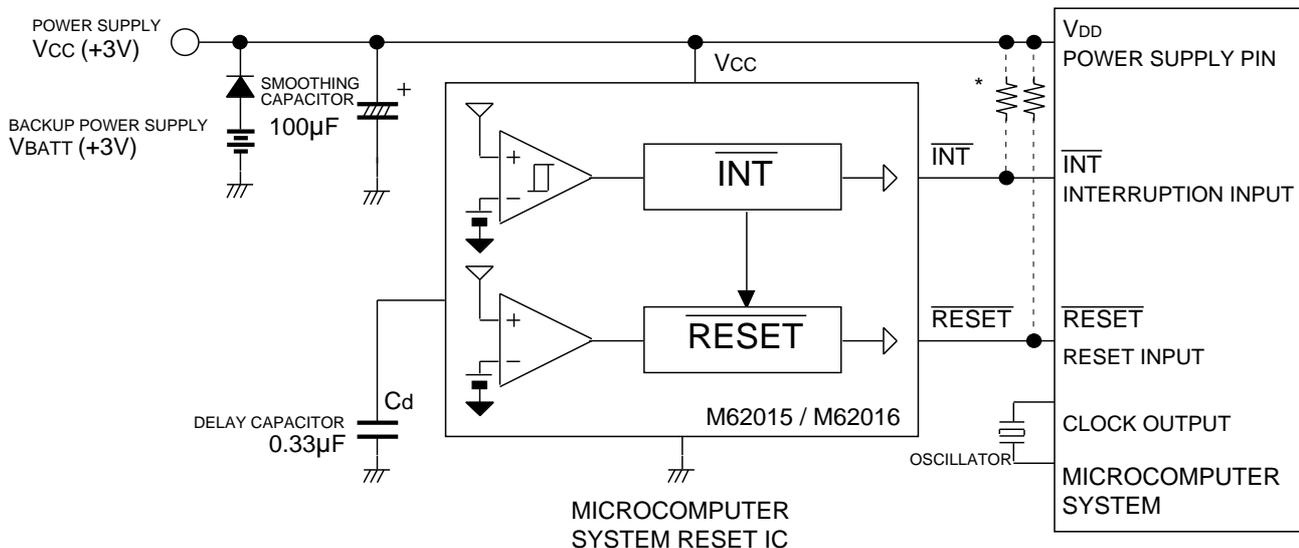
\* : A pull-up resistor is required only in the case of open-drain output.
