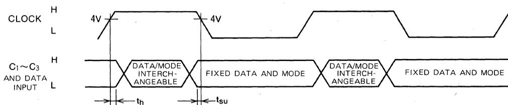
Note 4:  $C_1 \sim C_3$  and accept data (AD accept data) are interchangeable while the clock is set high.
