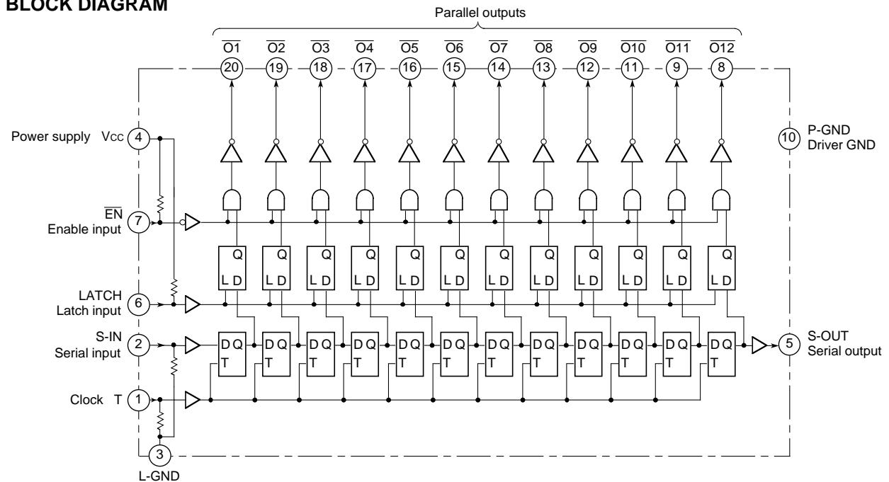
**Bi-CMOS 12-BIT SERIAL-INPUT LATCHED DRIVER**
