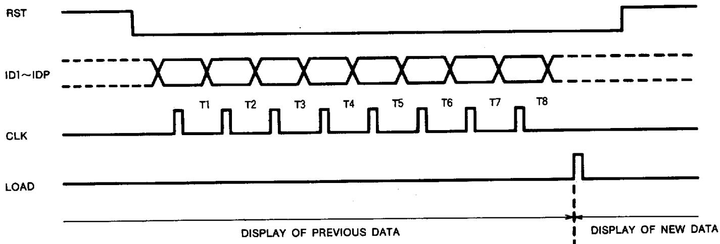
After the 8th clock input, the LOAD is valid only in the period while RST="L". Furthermore, if there is 9th CLK input before the LOAD input, the LOAD input is ignored.
