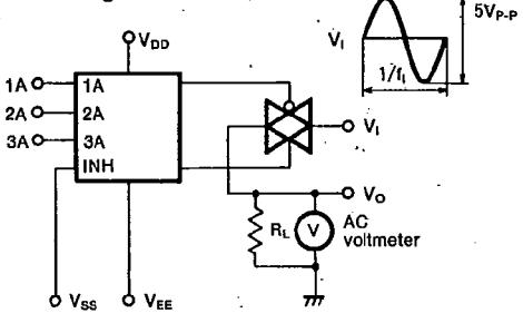
The feedthrough is taken as that frequency f<sub>I</sub> at which, using a sine-wave input of 2.5V<sub>p-p</sub>,  $20 \log_{10}(V_o/V_i) = -50$ dB. Refer to the function table for conditions of control Input A.**7 Crosstalk**
