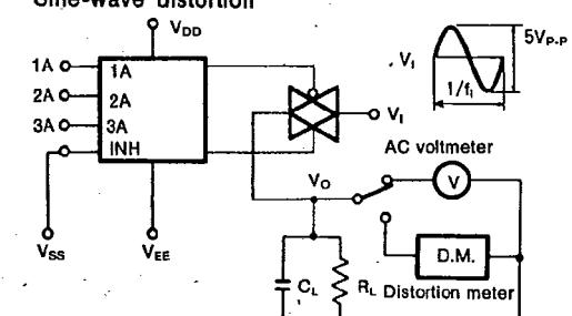
$f_{max(I/O)}$  is taken as that frequency  $f_i$  at which, using a sine-wave input of  $2.5V_{p-p}$ ,  $20 \log_{10}(V_O/V_I) \approx -3\text{dB}$ . Refer to the function table for conditions of control input A.
