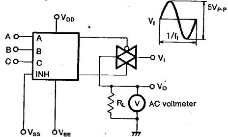
The feedthrough is taken as that frequency  $f_i$  at which, using a sine-wave input of 2.5V<sub>P-P</sub>,  $20 \log_{10}(V_o/V_i) = -50$ dB. Refer to the function table for conditions of control inputs A, B, and C.
