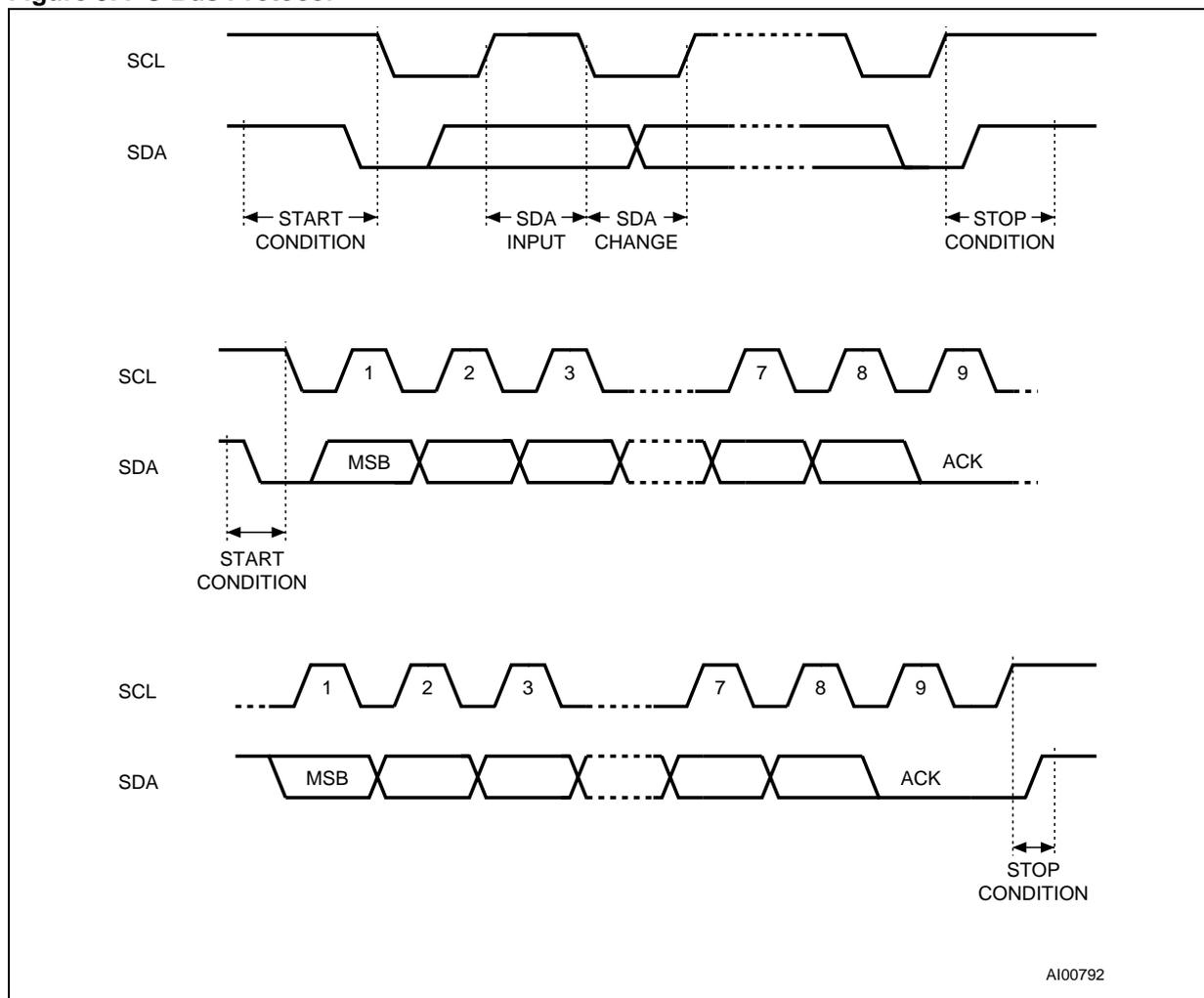
reads the data to be a receiver. The device that controls the data transfer is known as the master, and the other as the slave. A data transfer can only be initiated by the master, which will also provide the serial clock for synchronization. The memory device is always a slave device in all communication.
