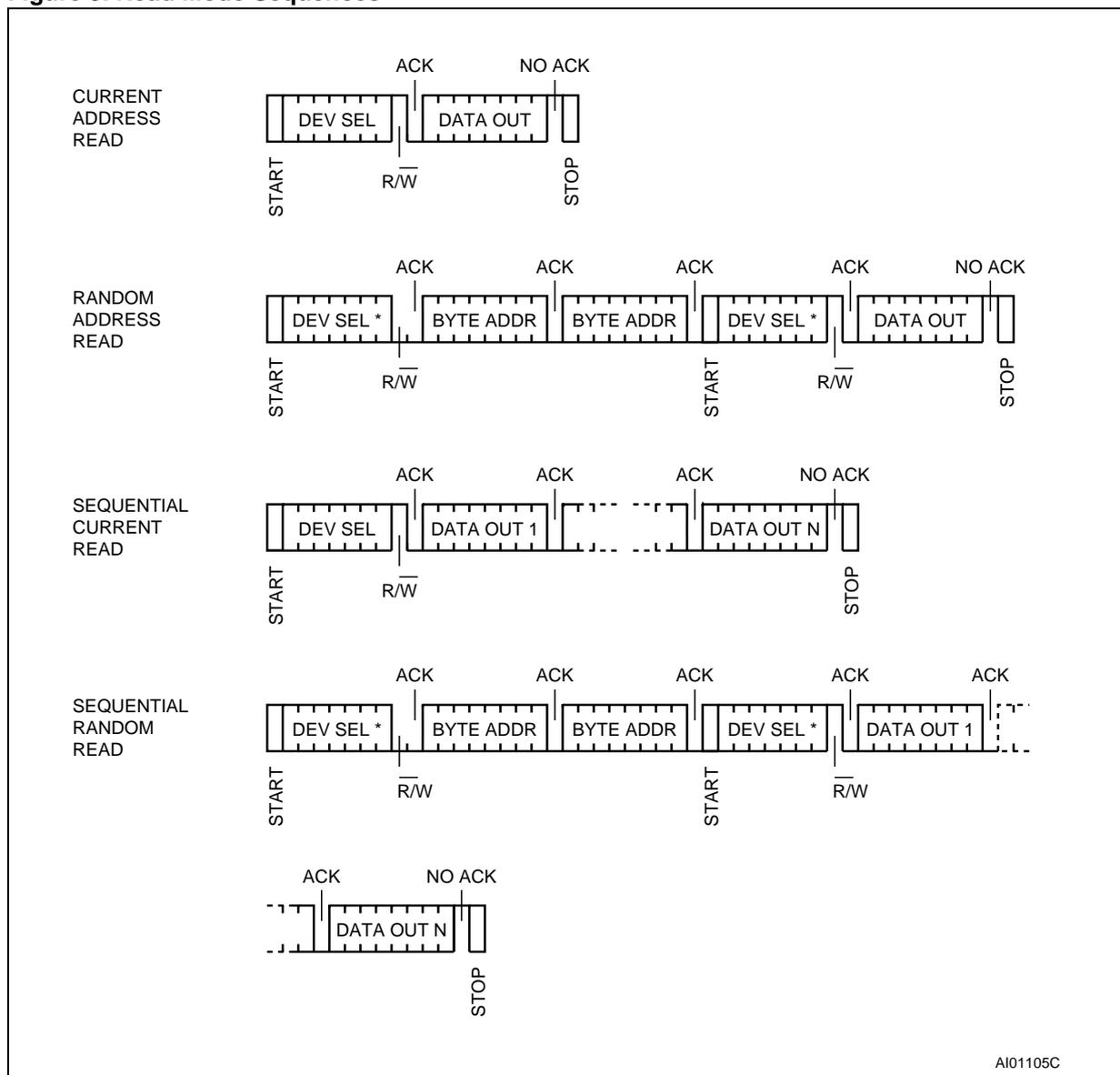
Note: 1. The seven most significant bits of the Device Select Code of a Random Read (in the 1<sup>st</sup> and 4<sup>th</sup> bytes) must be identical.
