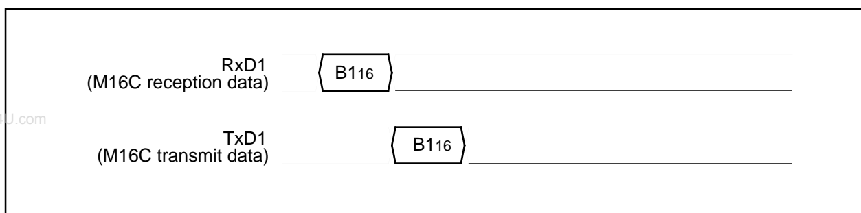
Figure 1.32.39. Timing of baud rate 19200
