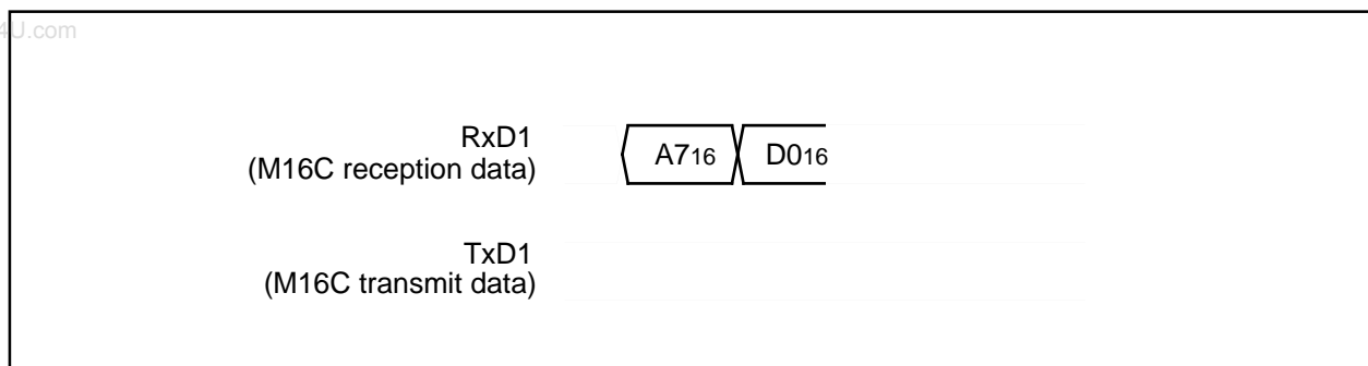
Figure 1.32.27. Timing for erasing all unlocked blocks
