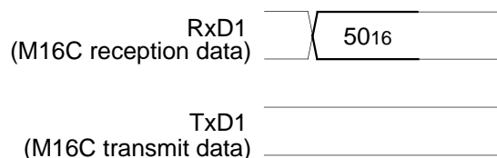
Figure 1.32.24. Timing for clearing the status register
