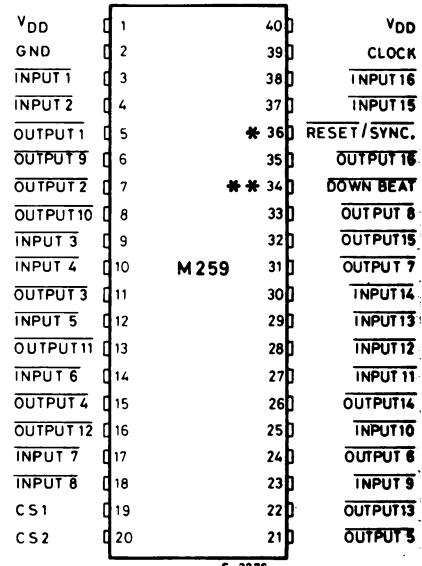
\* This is a bidirectional pin. Used as an input it allows the chip reset; used as an output it can reset other devices.
