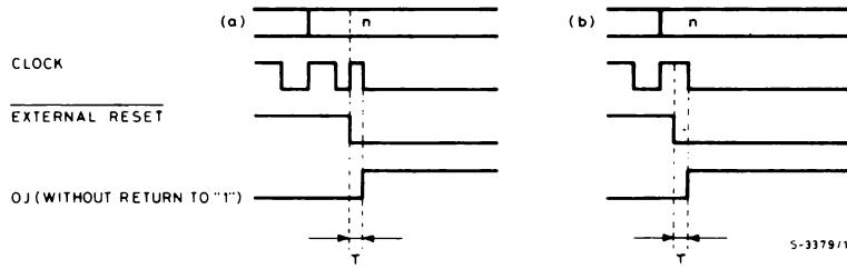
In both the cases the delay  $\tau$  (in the outputs without return to "1") is defined through the constant  $R1 C1 \geq 10 \mu\text{sec}$ .
