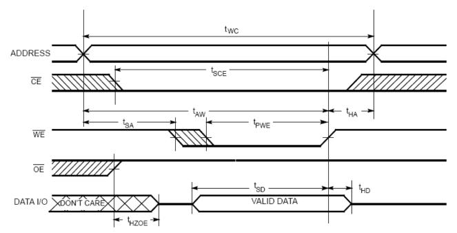
Switching Waveforms (continued) Write Cycle 2 ( $\overline{CE}$  Controlled) [10, 11, 15, 16, 17]
