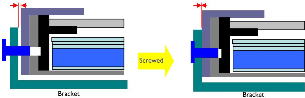
**9.6 Avoid scratching LCM, the rib on system front-cover should not exceed the bottom edge of LCM's front-bezel.**
