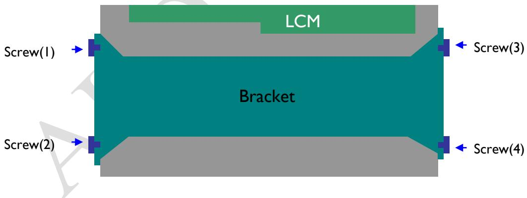
9.5 The system bracket and panel should be in parallel with having no gap after inserting screws.
