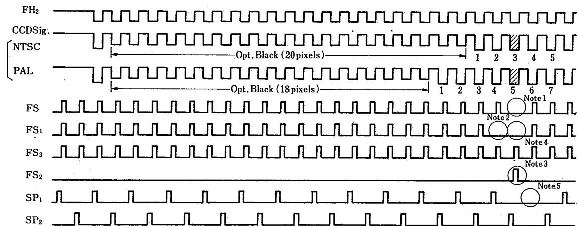
The LZ92B31 defect compensation IC in combination with a ROM recorded with defect pixel addresses will output the following pulses.
