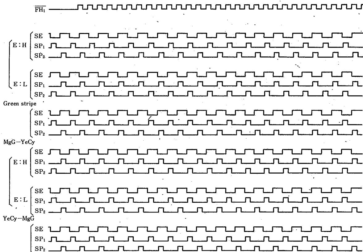
**Pulse output timing of FS, FS<sub>1</sub>, FS<sub>2</sub>, FS<sub>3</sub>, SP<sub>1</sub> and SP<sub>2</sub> for defect compensation**
