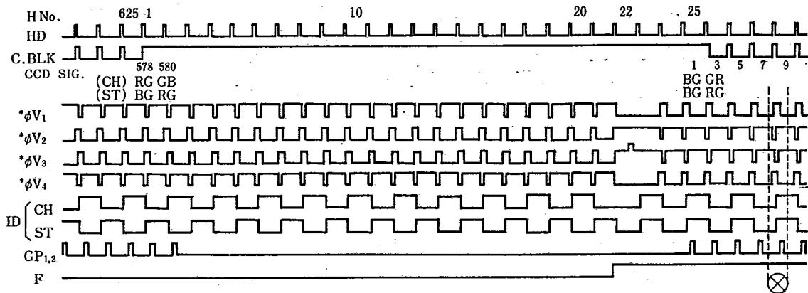
\*  $\phi$ V<sub>1</sub>- $\phi$ V<sub>4</sub> pulses apply to the CCD.
