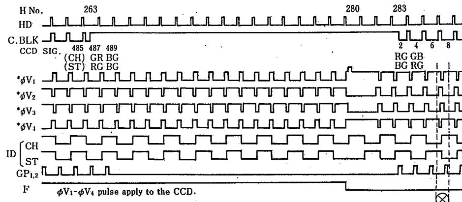
$\phi$ V<sub>1</sub>- $\phi$ V<sub>4</sub> pulse apply to the CCD.
