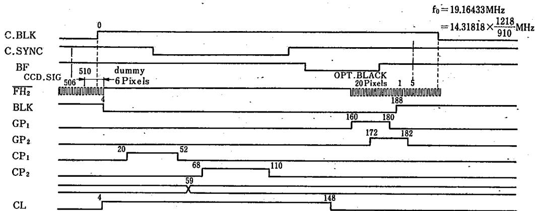
Field transfer (Enlarged timing of the area marked with  $\otimes$ )
