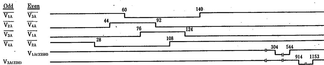
Timing Pulse Generator LSI for 2/3" CCD
