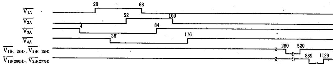
Frame transfer (Enlarged timing of the area marked with  $\otimes$ )
