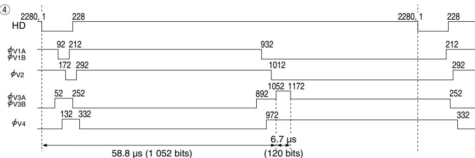
\* Keep over 2.2 µs when vertical transfer clock pulse is overlapping.
