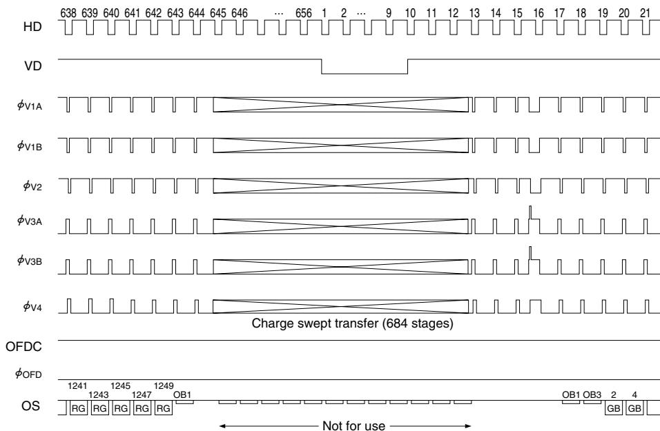
⑤ VERTICAL TRANSFER TIMING [FIELD ACCUMULATION MODE AT FIRST]
