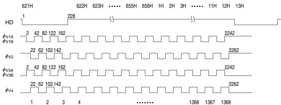
\* Keep over 1.1  $\mu$ s when vertical transfer clock pulse of charge swept transfer is overlapping.
