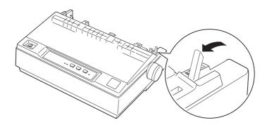
2. Release the sprocket units by pulling the sprocket locks forward.
