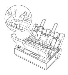
14. Slide the left edge guide to the center until it stops at the guide mark. Then slide the right edge guide to the opposite guide mark.
