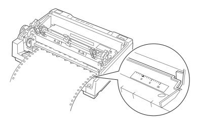
6. Slide the left sprocket unit so that its sprockets match the position of the holes in the paper and lock the unit in place. Then slide the right sprocket unit to match the width of your paper, but do not lock it. Move the paper support midway between the two sprocket units.
