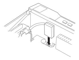
4. Slide the print head to the middle of the printer; then slide the plastic part on the color ribbon to the center of the cartridge.
