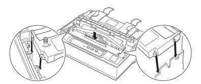
5. Use a pointed object, such as a ball point pen, to guide the ribbon between the print head and ribbon guide. Turn the ribbon tightening knob to help feed the ribbon into place; it should not be twisted or creased.
