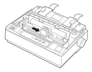
3. Turn the ribbon-tightening knob in the direction of the arrow to remove any slack from the ribbon so it is easier to install.
