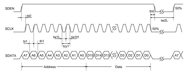
Data length : 24bit Clock frequency : 3MHz or les
