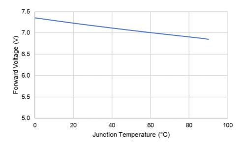
Fig.7 Forward Voltage vs Junction Temperature
