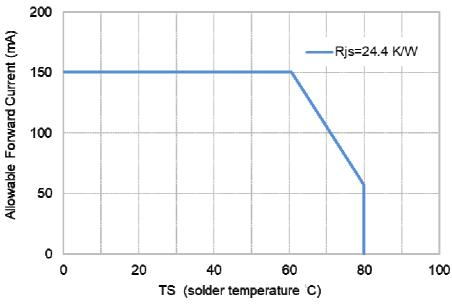
Fig 6. Forward Current Derating Curve
