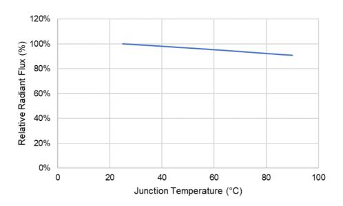
Fig.4 Relative Radiant Flux vs Junction Temperature
